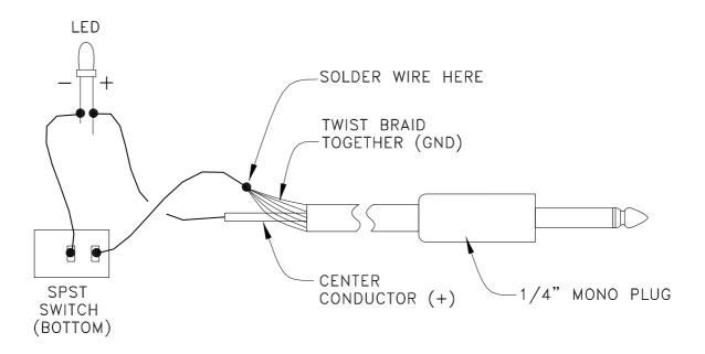
NOTES: ISOLATING SWITCH FROM ENCLOSURE IS NOT NECESSARY.
